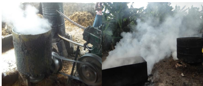
Figure 4: Gaseous emission sources from smallholder oil palm processing mill in Nigeria
